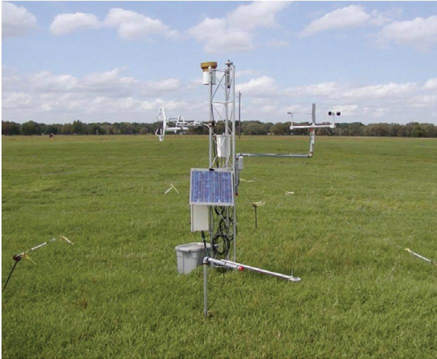
A typical grower weather station for use in the Florida Automated Weather Network cost-share program.
