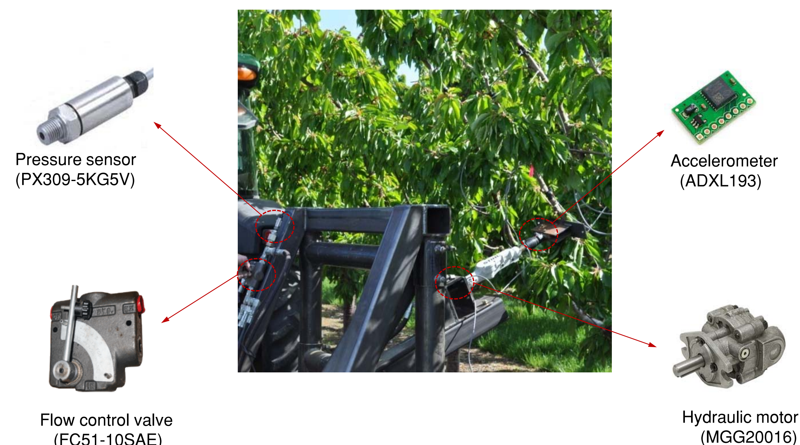
Fig. 3 Field tests in sweet cherry orchard using developed shaker system
