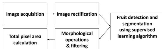
Fig. 5. Block diagram of image processing algorithm
