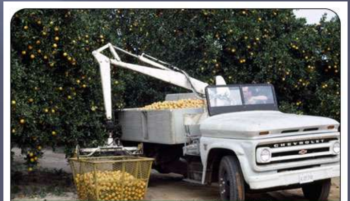
Bulk handling of processed citrus with metal baskets and the "Lightning Loader".
