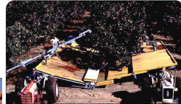
First generation CREC slider crank limb shaker catchframe harvest system.
